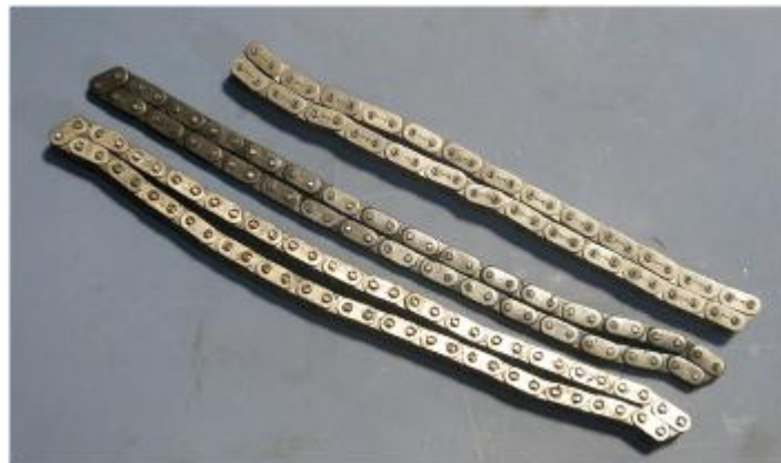
From top to bottom: Wrong duplex chain, original chain, and new duplex chain
